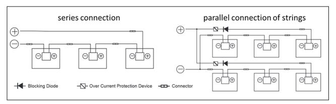
Suitable overcurrent protection measures (e.g. string cut-out) are required for the parallel connection of the modules. It must be ensured that the specified capacity regarding the return current IR of the datasheet will not be exceeded. If there are more than two parallel strings, string fuses and string diodes must be used.
