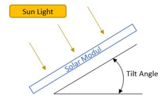
A module inclination of at least 10° is recommended. If the module inclination is less than 7.5°, sufficient cleaning must be ensured. Building regulations must be observed (in Germany maximum 75°).
