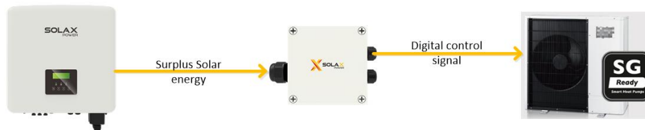
Figure 11: Adapter Box G2 to Heat Pump Connection Diagram
